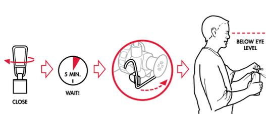
**NOTICE:** To transport the Fuel Bottle, the Pump may be left inside a depressurized Fuel Bottle. The Pump can also be removed and replaced with the Fuel Bottle Cap.
